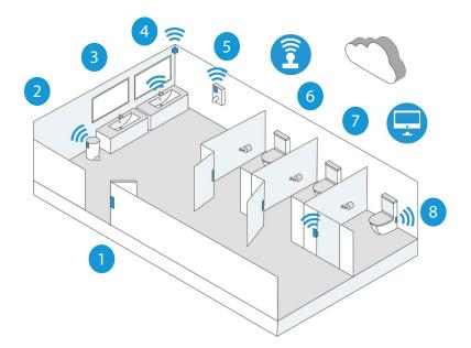
occupancy levels within the toilet area with the Netvox R718PQ Wireless Short-Range Occupancy Sensor. Offering state of the art infrared detection this smart device can pick up humans and animals at a range of 2m at a 72
